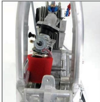
Also uses the supplied manifold adapter. Set adapter offset to the left with the throttle cable running between the frame spar and gas tank.
