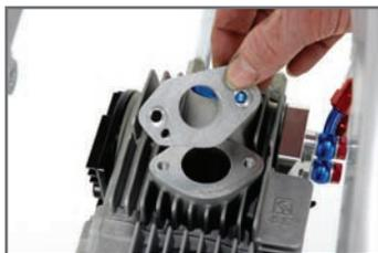
Use supplied manifold adapter to center the carburetor.
