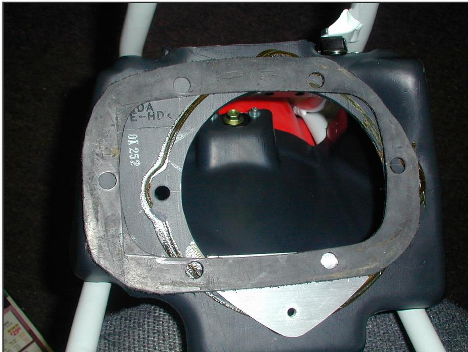
Step 4: Mark the inside of the template and the mounting holes.
