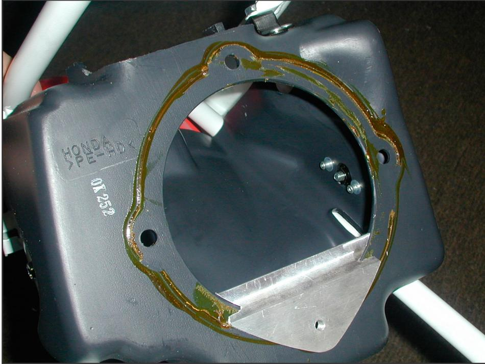
Step 3: Lay the template (of the XR200 airboot mount) on the airbox as shown.
